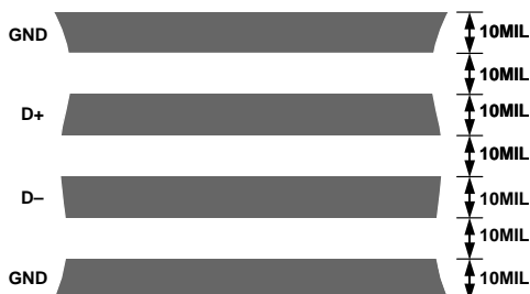
Figure 18. Arrangement of Signal Tracks
